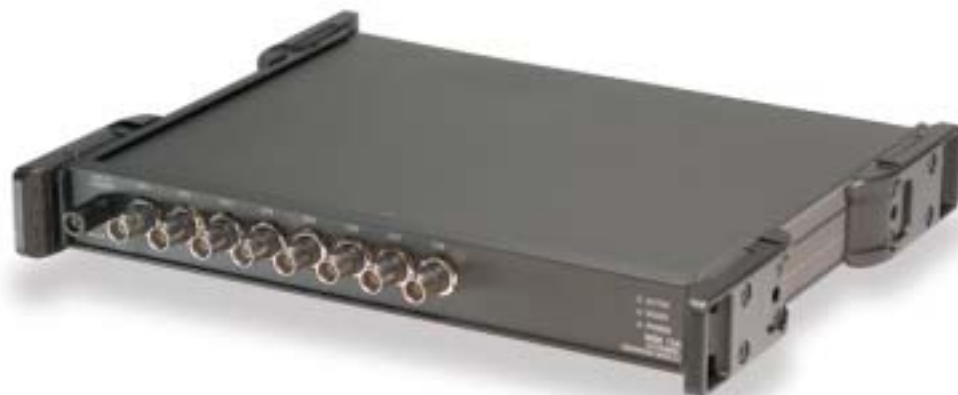
The WBK10A adds eight differential analog inputs to your WaveBook system
